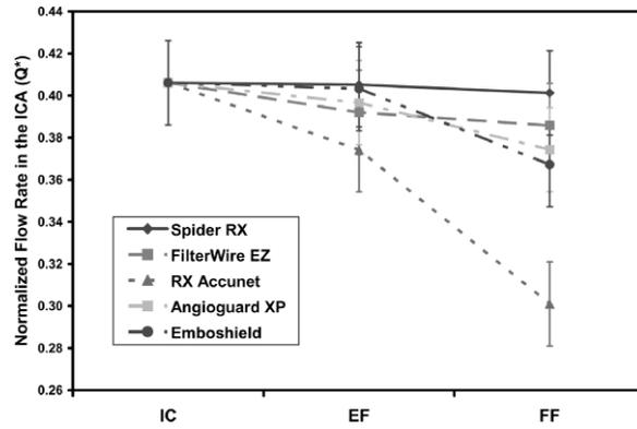
**Figure 5** ♦ Normalized volume flow rate with y error bars in the ICA. IC: initial condition (prior to device deployment), EF: empty filter condition (device deployed), FF: full filter condition (device filled with particles)
