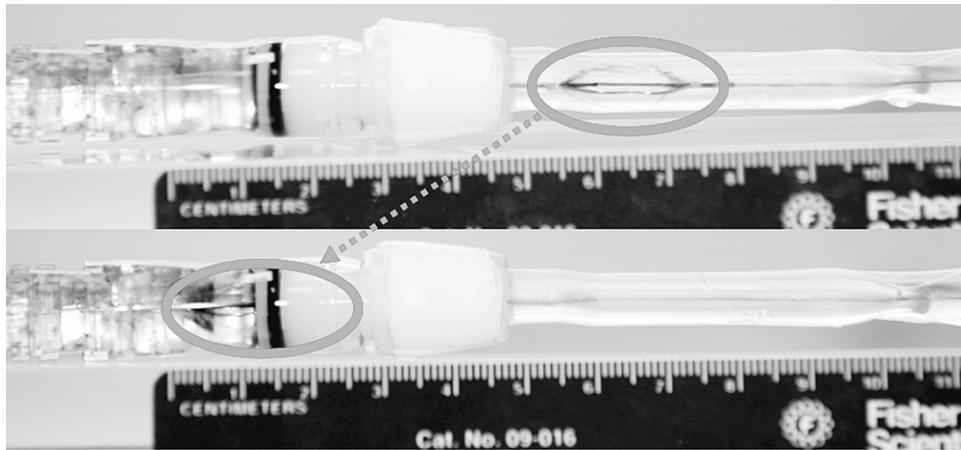
Figure 6 ♦ Distal migration of unclamped Emboshield device.
