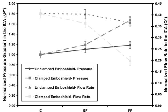
**Figure 7** ◆ Normalized pressure gradient and volume flow rate with y error bars in the ICA for the unclamped and clamped Emboshield guidewire. IC: initial condition (prior to device deployment), EF: empty filter condition (device deployed), FF: full filter condition (device filled with particles)
