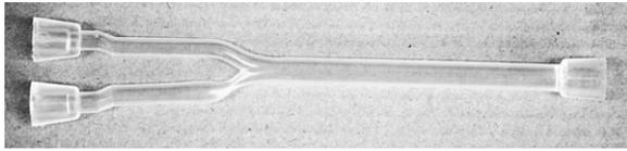
**Figure 2** ♦ Photograph of the symmetric 70% stenosed carotid bifurcation phantom.
