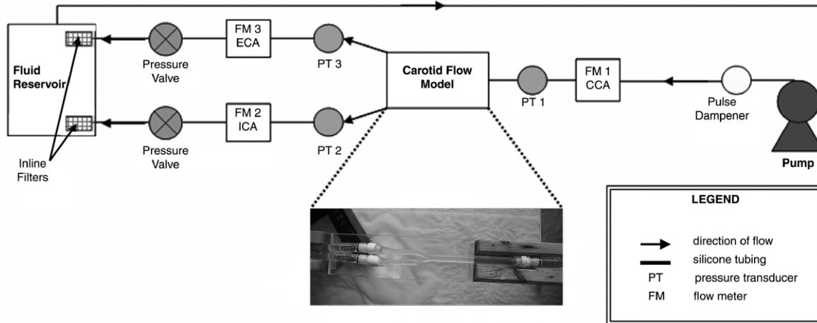
**Figure 1** ♦ Schematic of flow loop system with inset of carotid artery model.<sup>11</sup> CCA: common carotid artery, ICA: internal carotid artery, ECA: external carotid artery.
