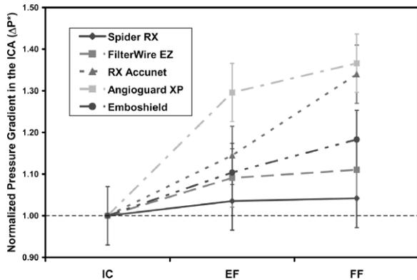
**Figure 4** ♦ Normalized pressure gradient with y error bars in the ICA. IC: initial condition (prior to device deployment), EF: empty filter condition (device deployed), FF: full filter condition (device filled with particles).
