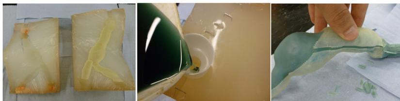
**Fig. 3** Process for the inner mold: silicone mold with the AM artery (left), filling the mold with liquid wax (center), and opening the AM artery to remove the wax mold (right)
