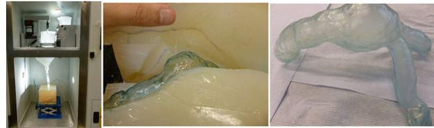
**Fig. 4** Vacuum casting process for the artery: silicon mold with the wax mold inside ready for casting the PUR resin (left), opening the mold to remove the artery (center), and the final artery replica (right)
