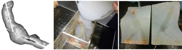
**Fig. 2** Partition lines for the artery, with their proper connector pins (left), AM artery within the mold and filling the frame with silicon (center), and the final outer mold once cut open (right)
