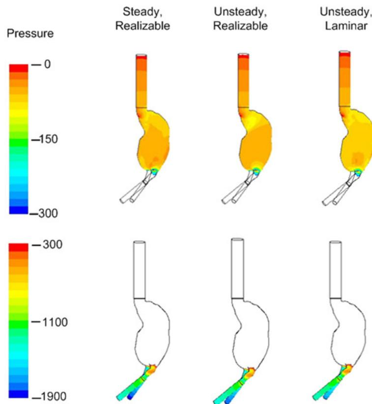
Figure 8. CFD-predicted pressure field in the model without ILT. Computations using three different models: (A) steady  $k-\varepsilon$  Realizable, (B) unsteady  $k-\varepsilon$  Realizable and (C) unsteady laminar.
