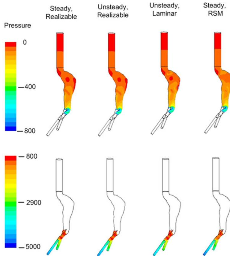
Figure 7. CFD-predicted pressure field in the model with ILT. Computations using four different models: (A) steady  $k-\epsilon$  Realizable, (B) unsteady  $k-\epsilon$  Realizable, (C) unsteady laminar and (D) steady RSM.
